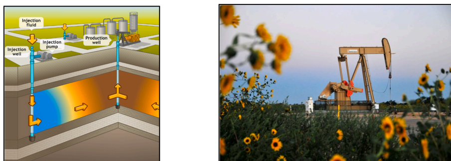
Fig. 3. Schematic of traditional oil recovery from an oil field where water or natural gas is injected behind the oil to push it toward a collecting well.
